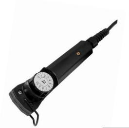
The "Dog bone" style remote control MMA offers stepless adjustment of the weld current. The adjustment knob can be accessed from both sides making the remote control ideal for both left and right hand operation. The minimum current, as a percentage of the set weld current, can be adjusted in the power source allowing for both Fine and Coarse setting of the current. For more information please refer to the power source user manual.
