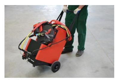
Portable hydraulic power pack with shelf for puncher transport.
